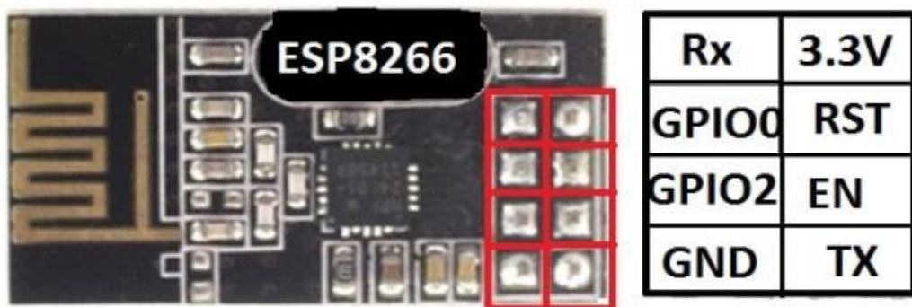
Figure 24: ESP8266 Pin diagram
