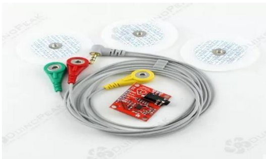
Figure 11: ECG Sensor Module (Ad-8232) [40] Figure 12 : Sensor Pad location on Body[40]
